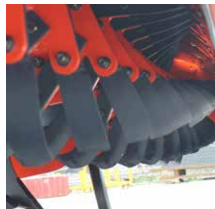
Version with a rotary cultivator for clay soils.
