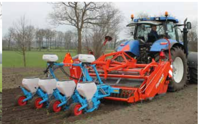
Additional roller for a sowing bed that holds moisture better.
