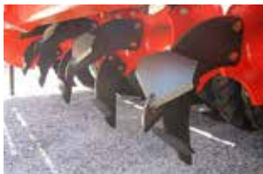
The spader blades are attached with shearing bolts
