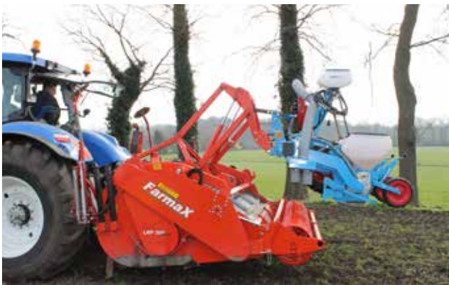
A top-mounted lift to combine with a sowing machine.
