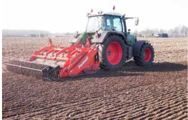
Additional roller for a sowing bed that holds moisture better.
