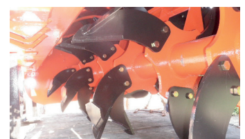
Attachment with shear bolts
