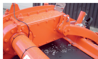
Intermediate drive for narrow transport width
